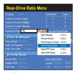
The Rear-Drive Ratio is the numerical gear ratio of the front or rear driving axle, depending on whether the vehicle is front- or rear-wheel drive. This ratio indicates the number of turns the drive-shaft (or pinion gear) rotates for each revolution of the rear wheels.
