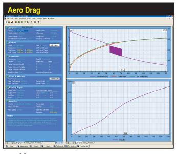
Total Drag, as displayed in the DragSim (lower graph), is the force from wind and rolling resistance that resists forward motion. Notice how Drag increases as this Top Fuel dragster approaches 300mph. Nearly 5000 pounds of force are resisting forward movement (due, in part, to a high-downforce wing model used by the DragSim when modeling 200+mph vehicles).
