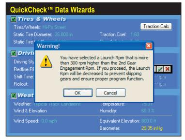
(**Torque Converter** shift times are set to zero, since power flow to the driving wheels is not interrupted during a shift). During the **Shift Time** the driveline is effectively in "neutral," sending the engine to the redline and the acceleration to zero. When the shift time has elapsed, the next gear is engaged and the vehicle continues to accelerate.
