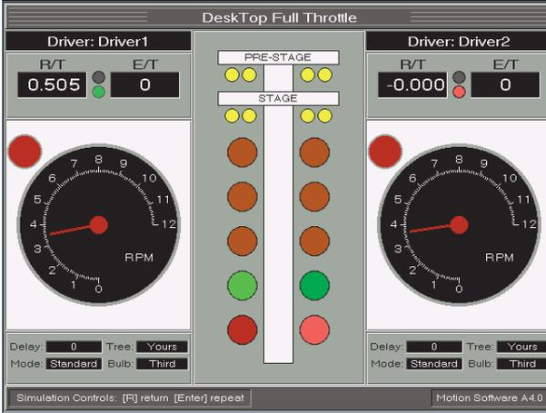
The *DeskTop Full Throttle Reaction Timer* software incorporates precision starting-line, shifting, and top-end simulations. Using basic vehicle parameters and performance data from the *DeskTop Drag* or *DragSim*, Full Throttle will simulate the driving characteristics of the vehicle at the starting “tree,” and throughout the 1/8- or 1/4-mile. Driver input is logged and analyzed, permitting anyone to improve their starting-line and shifting
