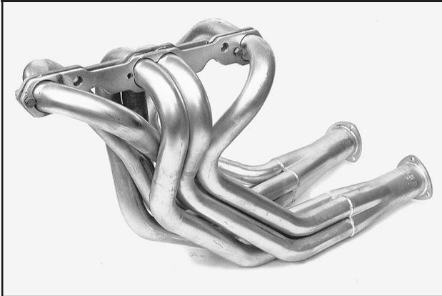
Typical large-tube headers are designed for high-performance street and racing applications in mind. The better pieces have 3- to 4-inch collectors and 1-3/4- to 2-3/8-inch primary tubes (depending on whether they were designed for smallblocks or bigblocks).
