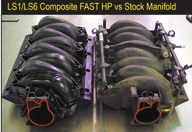
have been shown to add from 3% to 12% more power with very little sacrifice in bottom-end torque. You can test a performance design with the **LS1/LS6 HP Runner/Mod** induction selection in DynoSim5. This induction model was based on the FAST™ manifold for the same engine.
