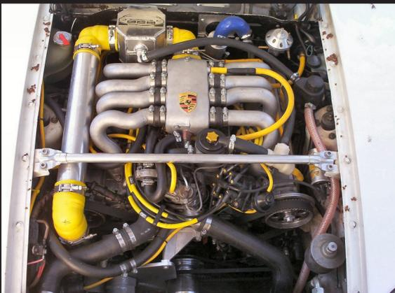
The *Long-Tubing Runners, Common-Plenum, Max-Flow* selection models manifold designs used on high-performance engines or in racing applications, like this Porsche 928 V8. The large runner cross-sectional areas ensure cylinder filling at high engine speeds, however, the additional runner and plenum volume can reduce torque at low rpm, offset somewhat, in this case, by the length of the runners.
