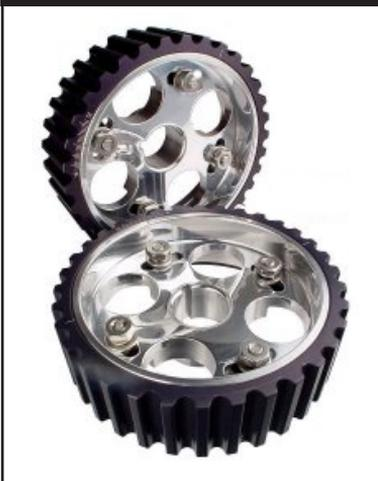
In DOHC engines, like the Honda VTEC and many other "sport-compact" engines, where separate cams are used for the intake and exhaust lobes, the advance/retard values can be set independently for the intake and exhaust lobes. In the real world, this same modification is easily accomplished with adjustable cam sprockets, like these from ZEX. Adjustable timing sprockets can also compensate for milled deck and head surfaces that can often result in retarded cam timing.
