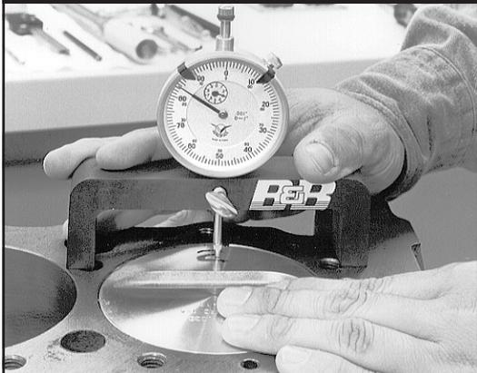
Use a dial indicator and stand to measure how far down the bore the piston is positioned at TDC. Enter a positive number for “down-the-bore” distances and a negative number if the piston protrudes above the deck surface. A typical value might be +0.040, indicating that the piston comes to a rest at TDC 0.040-inch below the deck surface.
