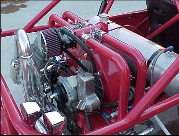
The *Long-Tubing Basic OEM* manifold selection models induction systems often used on a flat-four and flat-six engines, like the VW and lower-performance opposed-six Porsche powerplants. The length of the runners and their relatively small diameters optimize torque output, but restrict airflow at higher engine speeds.
