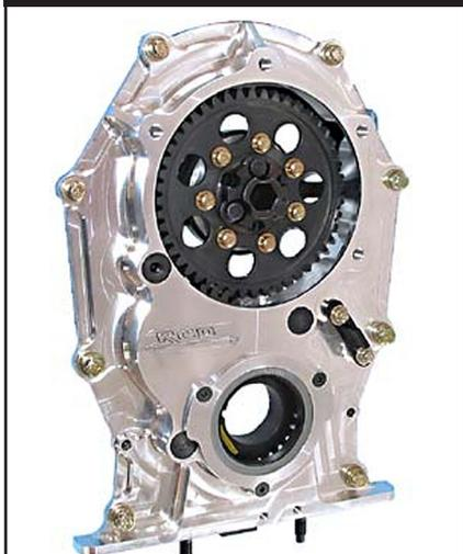
*Race Car Dynamics* manufacturers this beefy adjustable cam drive that makes it relatively easy to vary cam advance and retard on engines with single camshafts. Most cam manufacturers recommend installing their camshafts “heads-up,” or at the recommended specifications. In addition, advancing or retarding the cam will alter piston-to-valve running clearance. Make sure you have thoroughly tested the engine at cam advance/retard positions before you use it for tuning purposes.
