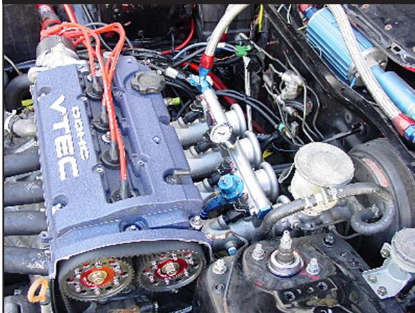
For naturally-aspirated, professional racing applications, individual- (or isolated) runner (I.R.) induction systems, with separate tubes containing their own throttle plates for each cylinder, offer the ultimate in flow potential and peak power at high engine speeds.
