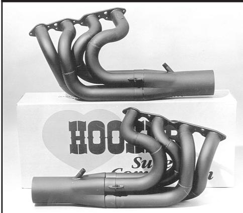
Large-tube stepped headers have large-diameter primary tubes with several transitions to slightly larger tubing diameters. These “steps” can reduce pumping work and improve horsepower on large displacement and/or high-rpm applications. These Hooker ProStock BB Chevy headers have 2-3/8-inch primary tubes that step to 2-1/2-inch as they reach the 4-1/2-inch collectors.
